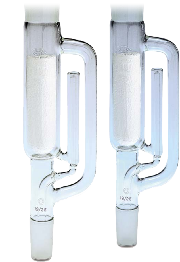
Extraction thimbles in Soxhlet extraction apparatus
